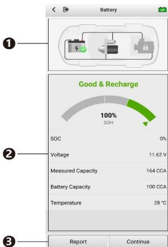
Figure 4-6 Sample Battery Test Result Screen
