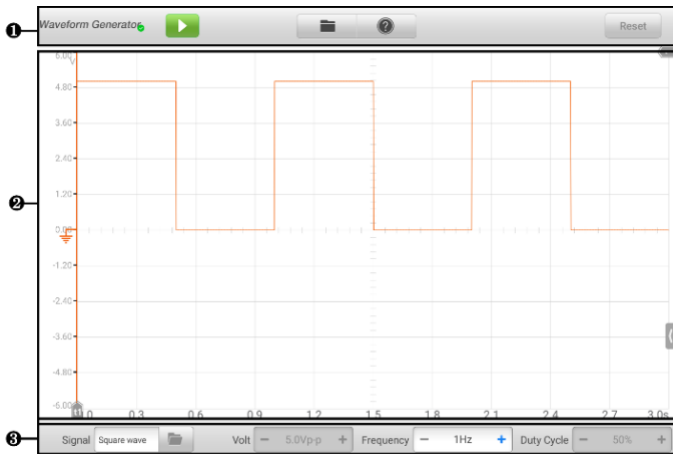
Figure 7-85 Waveform Generator Menu Screen
