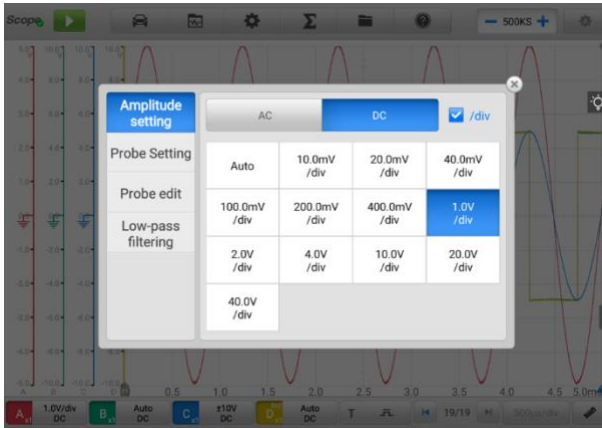
Figure 7-42 Amplitude Setting Screen (DC 1.0 V/div)
