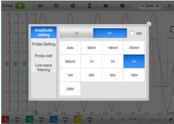
Figure 7-41 Amplitude Setting Screen (DC 5 V)
