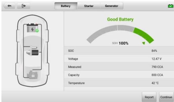
Figure 8-6 Battery Test Results Screen
