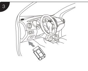
• Insert the MaxiVCI V150 into the vehicle's DLC, which is generally located under the vehicle dashboard.
