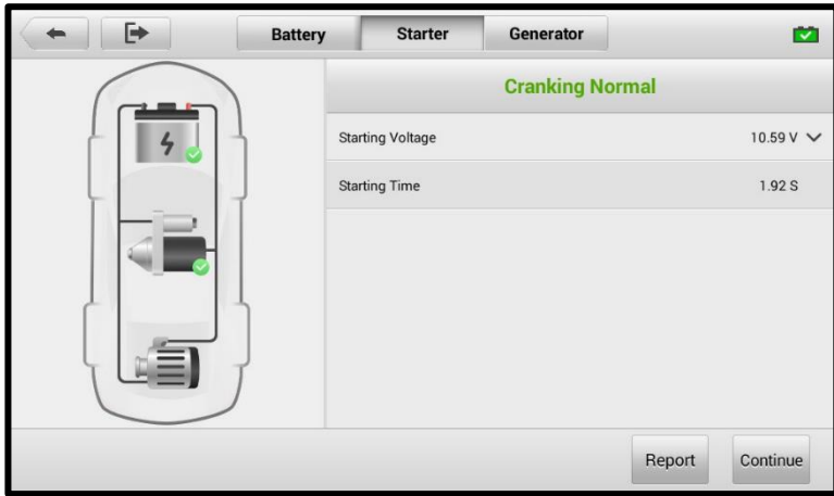
Figure 12-8 Starter Test Result Screen
