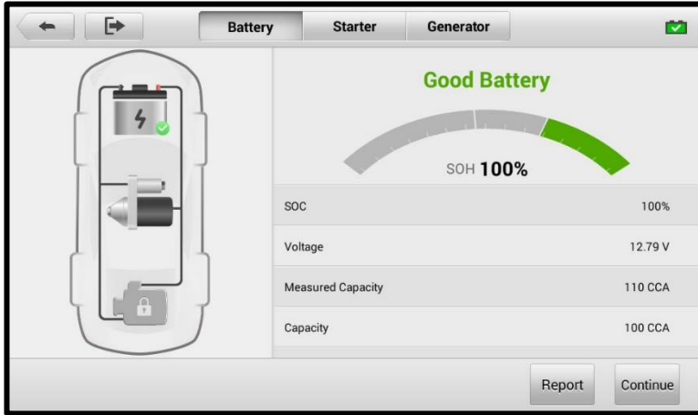
Figure 12-7 Battery Test Results Screen
