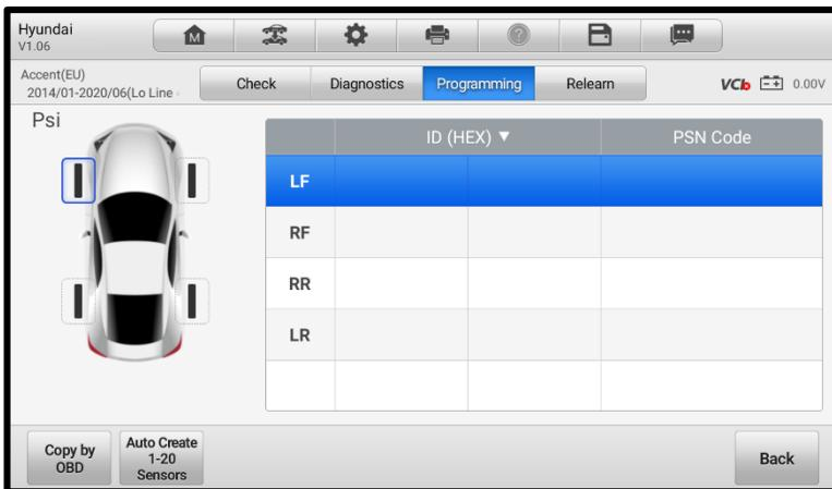
**Figure 6-23 Programming Function Screen**
