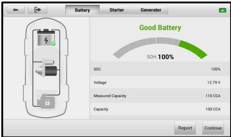
Figure 10-7 Battery Test Results Screen
