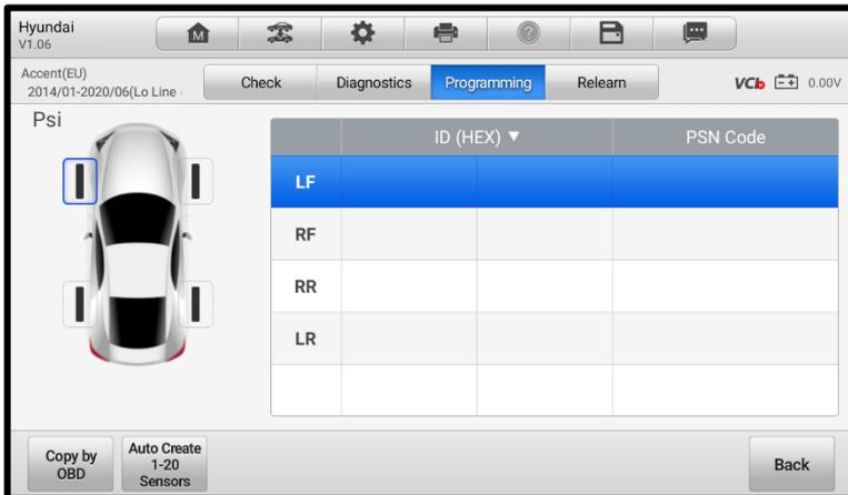
Figure 6-23 Programming Function Screen
