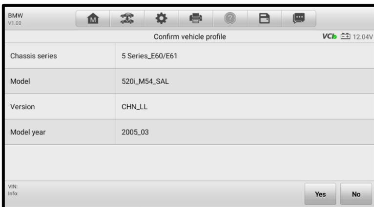
**Figure 4-4 Vehicle Profile Screen**
