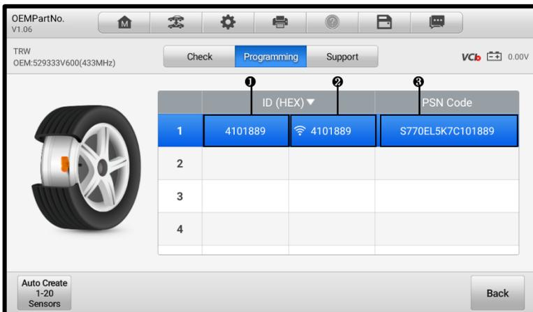
**Figure 6-40 Programming Screen via OEM Part NO.**
