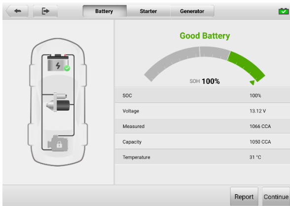
Figure 6-4 Battery Test Results Screen
