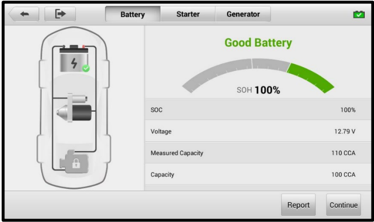
Figure 10-7 Battery Test Results Screen
