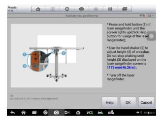
Figure 4-12 Calibration Frame Setup Instructions
