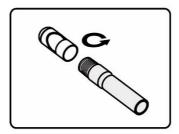
2. Screw the thread part of the accessory over the imager head to tighten the accessory.
