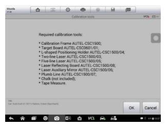
Figure 4-11 Tablet Displays Required Calibration Tools
