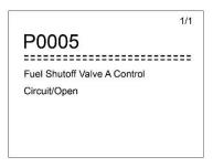
Figure 4-6 Sample DTC Screen
