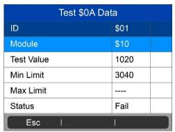
Figure 4-24 Sample Test Data Screen
