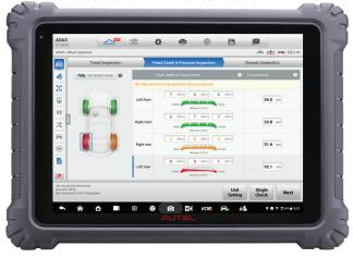
Inspect, image, and document a vehicle's brakes, suspension, and steering component condition and measure tire wear with the laser-enabled Autel TBE200.
