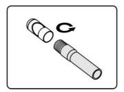
2. Screw the thread part of the accessory over the imager head to fix the accessory.
