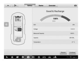
Figure 17-6 Sample Battery Test Results Screen
