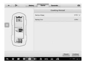
Figure 17-7 Sample Starter Test Result Screen
