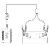
Figure 17-3 Sample Battery Tester Connection 2
