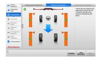
Figure 5-37 Start Rolling Compensation 1 (Using Rim Clamp)
