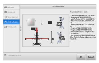
Figure 6-3 Prepare ACC Calibration Tools
