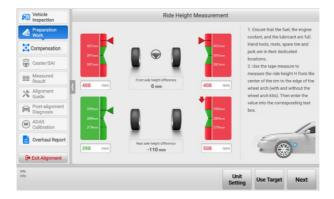
Figure 5-31 Measure Ride Height with Tape 1
