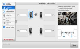
Figure 5-35 Measure and Input Tilt Angles
