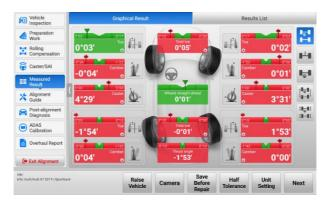
Figure 10-70 Measured Result (Full Tolerance) Screen
