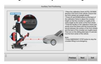
Figure 10-57 Auxiliary Tool Positioning 3
