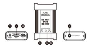
Figure 2-5 MaxiFlash VCI Programming Device
