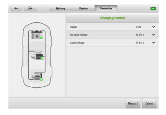
Figure 9-9 Generator Test Results Screen
