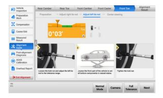
Figure 5-61 Adjust Left Tie Rod
