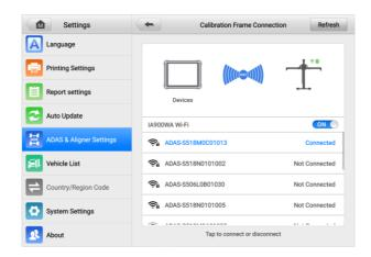
Figure 10-7 Connecting IA900WA to MaxiSys Tablet 2
