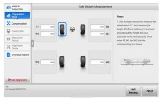
Figure 5-32 Measure Ride Height with Tape 2
