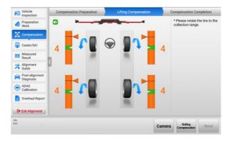
Figure 5-43 Start Lifting Compensation 1 (Using Rim Clamp)
