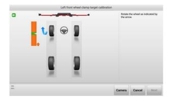
Figure 10-36 Start Calibration (Using a Vehicle) 3
