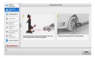
Figure 5-33 Install Ride Height Target
