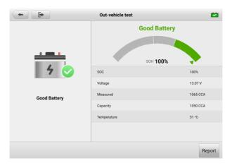
Figure 9-11 Out-vehicle Test Results Screen
