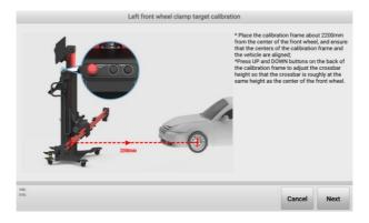
Figure 10-33 Calibration Preparation (Using a Vehicle) 2
