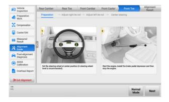
Figure 5-59 Front Toe Adjustment Preparation
