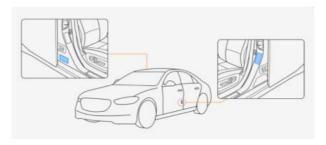
Figure 5-17 Standard Tire Pressure Value Location
