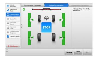
Figure 5-40 Start Rolling Compensation 4 (Using Rim Clamp)
