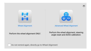
Figure 5-1 Wheel Alignment Function Entrance Screen
