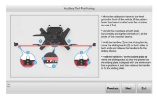
Figure 10-55 Auxiliary Tool Positioning 1
