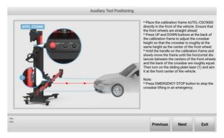
Figure 10-48 Auxiliary Tool Positioning 3
