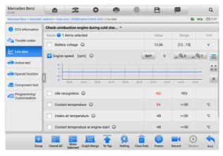
Figure 4-15 Waveform Graph Mode Screen
