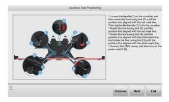
Figure 10-47 Auxiliary Tool Positioning 2
