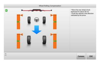
Figure 10-50 Wheel Rolling Compensation 1
