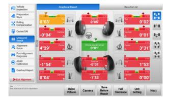
Figure 10-69 Measured Result (Half Tolerance) Screen
