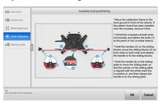
Figure 6-5 Position Auxiliary Tools for Calibration
