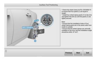
Figure 10-49 Auxiliary Tool Positioning 4
