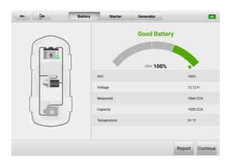
Figure 9-7 Battery Test Results Screen
