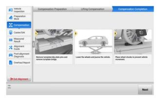
Figure 5-47 Complete Lifting Compensation (Using Rim Clamp)
