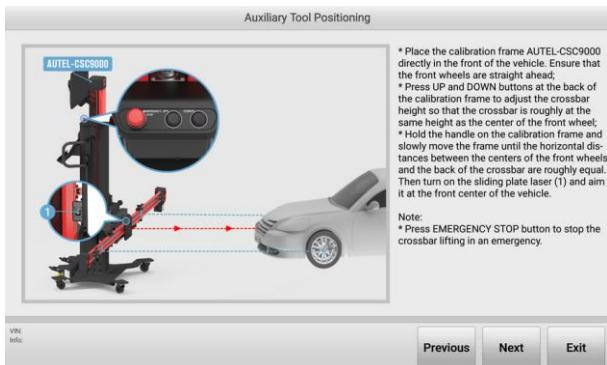
**Figure 10-57 Auxiliary Tool Positioning 3**
