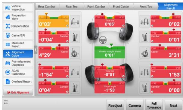
**Figure 5-58 Alignment Result Screen**
