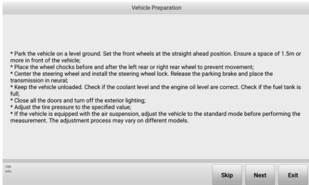
**Figure 10-54 Vehicle Preparation Guide**
