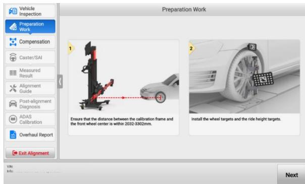
**Figure 5-33 Install Ride Height Target**
