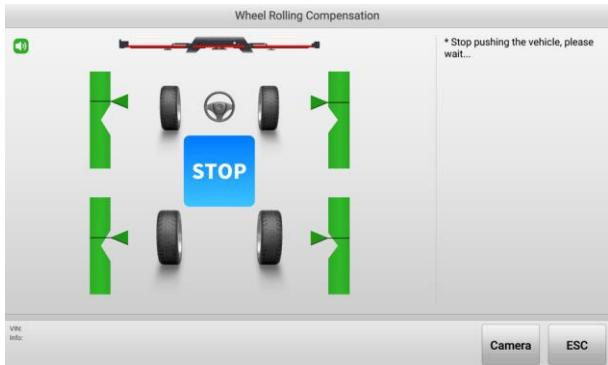
**Figure 10-51 Wheel Rolling Compensation 2**
