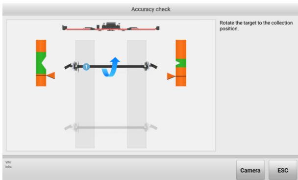
**Figure 10-42 Accuracy Check Screen (Using a Calibration Bar) 4**
