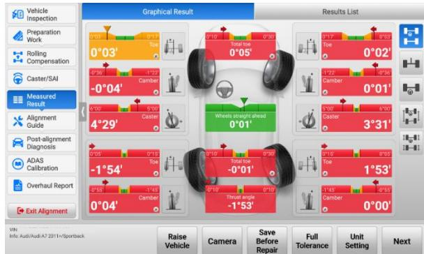
**Figure 10-69 Measured Result (Half Tolerance) Screen**
