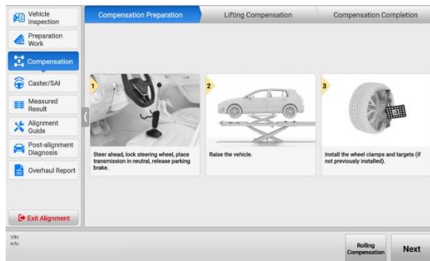
Figure 5-42 Lifting Compensation Preparation (Using Rim Clamp)
