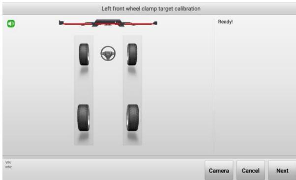
**Figure 10-35 Start Calibration (Using a Vehicle) 2**
