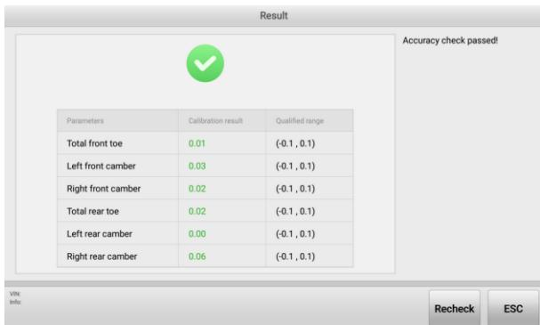
**Figure 10-44 Accuracy Check Result Screen**
