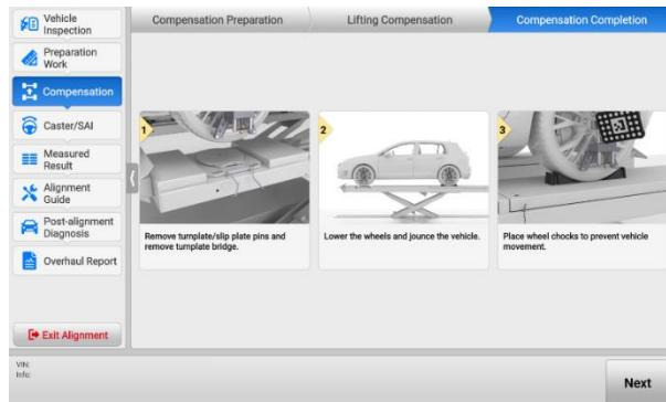
**Figure 5-47 Complete Lifting Compensation (Using Rim Clamp)**
