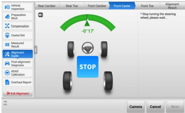
**Figure 5-64 Steering Wheel Adjustment**
