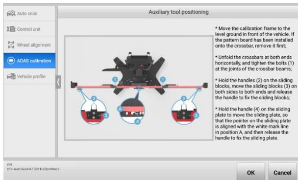
Figure 6-5 Position Auxiliary Tools for Calibration
