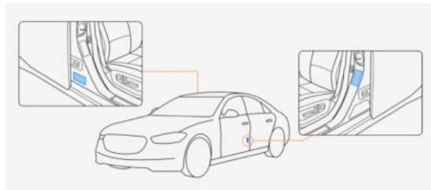
**Figure 5-17 Standard Tire Pressure Value Location**
