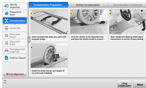
**Figure 5-36 Rolling Compensation Preparations (Using Rim Clamp)**
