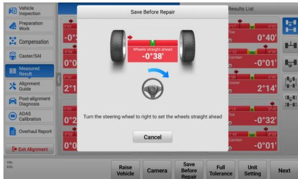
**Figure 10-67 Save Before Repair Screen 1**
