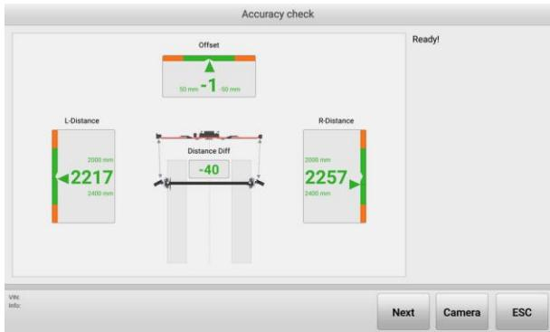
**Figure 10-41 Accuracy Check Screen (Using a Calibration Bar) 3**
