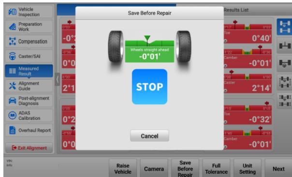
**Figure 10-68 Save Before Repair Screen 2**
