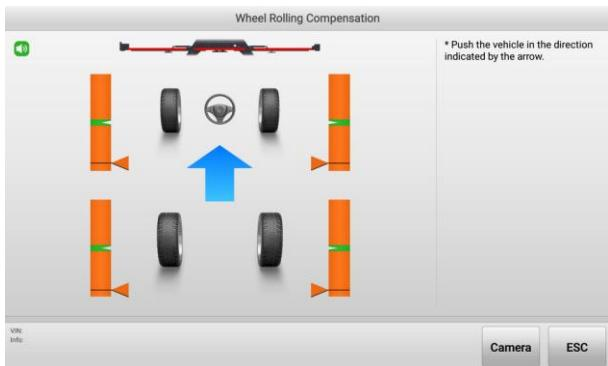
**Figure 10-52 Wheel Rolling Compensation 3**
