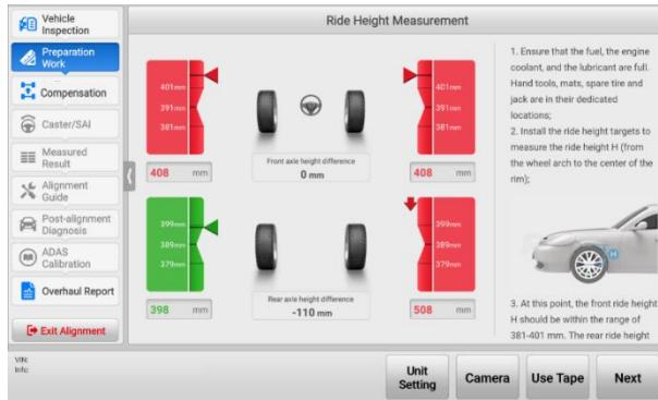
**Figure 5-34 Measure Ride Height with Ride Height Target**
