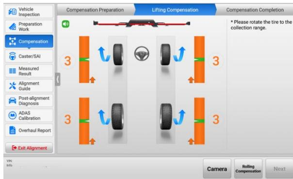
**Figure 5-44 Start Lifting Compensation 2 (Using Rim Clamp)**
