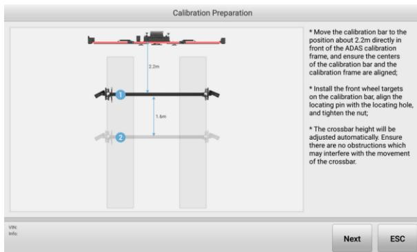
**Figure 10-17 Aligner Calibration Preparation**
