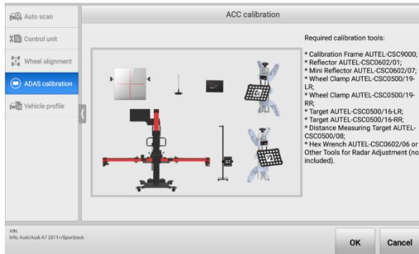
Figure 6-3 Prepare ACC Calibration Tools
