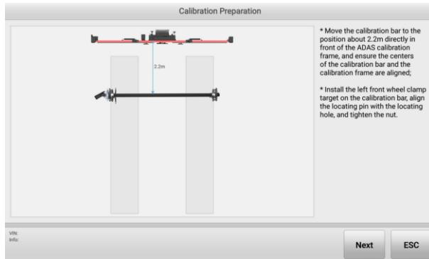
**Figure 10-25 Calibration Preparation (Using a Calibration Bar)**
