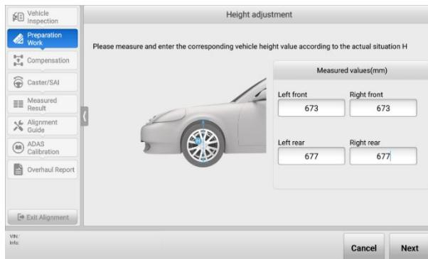
**Figure 5-28 Height Adjustment Screen 3**
