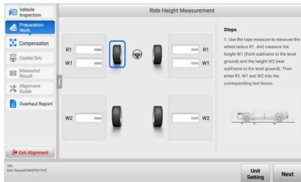
**Figure 5-32 Measure Ride Height with Tape 2**
