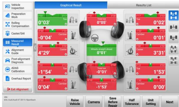
**Figure 10-70 Measured Result (Full Tolerance) Screen**
