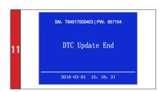
Downloaded software will overwrite and replace existing software on the tool . The message "Update End" will display on the tool once completed.
