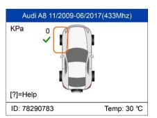
Press [?] to trigger the sensors.
