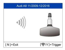
Press **Y** or **Trigger** to trigger the sensor.
