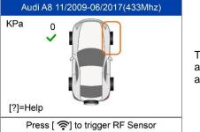
The next sensor is waiting to be activated. Press Trigger to scan all the sensors one by one.
