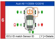
Green signal and OBD icons: the ECU ID matches Sensor ID. Red signal and OBD icons: the ECU ID does not match Sensor ID
