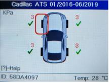
Picture 1 Picture 2 Follow the instruction to connect TS508 to the vehicle's DLC and then tap "Continue" to read IDs from ECU. Results will be displayed a few moment later, see picture 3. Before doing any relearn operation, the data of Step 1 and Step 2 will be recorded as the "Initial customer record".
