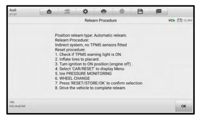
Figure 4-12 Relearn Procedure for Indirect TPMS
